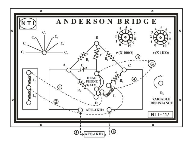
Fig. (2) Connections for ANDERSON BRIDGE
