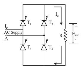
Fully-controlled bridge -circuit with resistive-load
