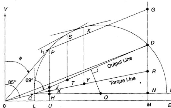
Fig. – ‘F’ : Circle diagram of an induction motor.
