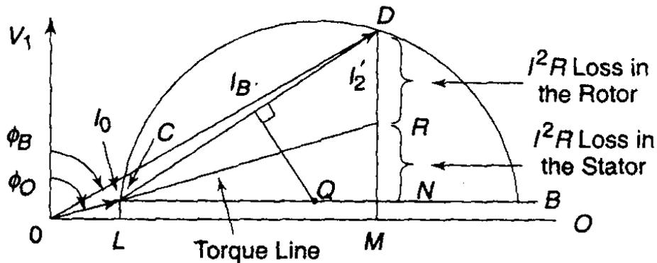
**Fig. - 'D' : Circle diagram of an induction motor .**
