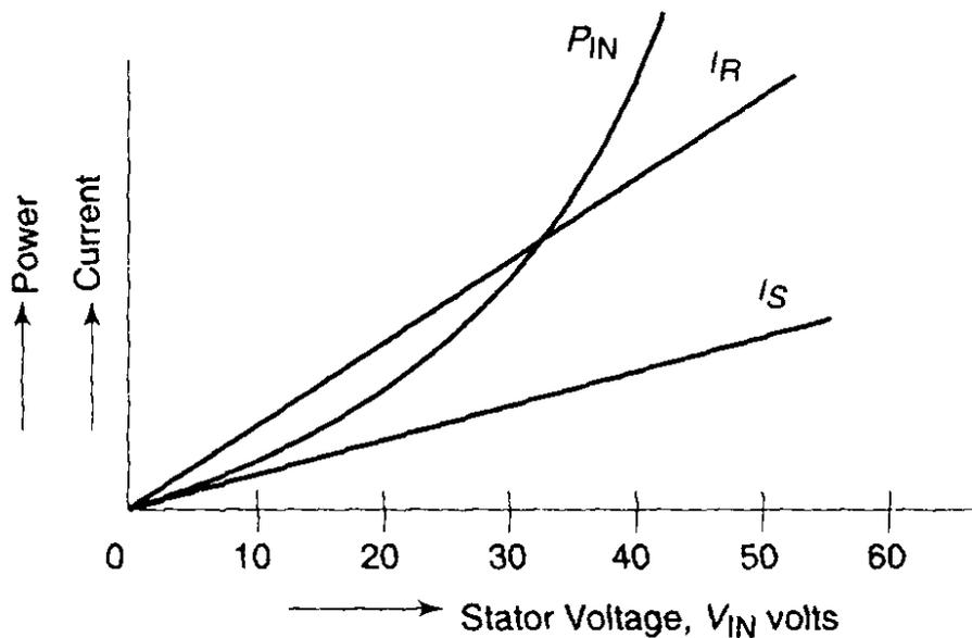
*Fig. – 'C' : Effect of exchange of stator applied voltage on power input, rotor and stator current .*
