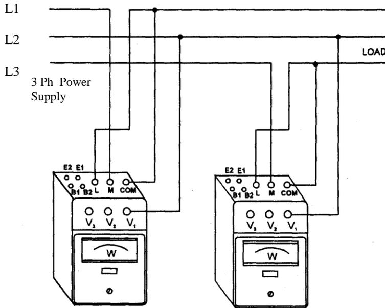
The three-phase power measurement is conducted by connecting two wattmeters, as shown in above Fig. The power value is indicated by the algebraical addition of the indication value on the two wattmeters. When the power factor of the circuit being measured is greater than 50%, both meters will indicated “positive” values. The total load power is then calculated by the addition of these two values.
