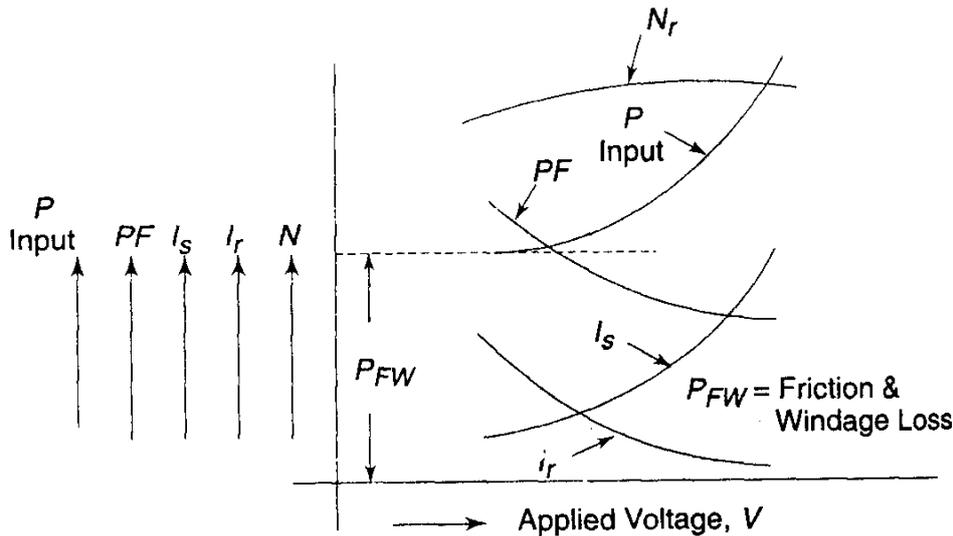
**Fig – ‘A’ : Effect of change of applied voltage on speed, Rotor current, Stator Current, Power factor and power input of an induction motor running on no-load.**
