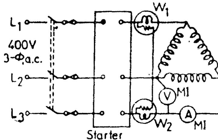
**STEPS FOR PERFORMING NO LOAD TEST :**
