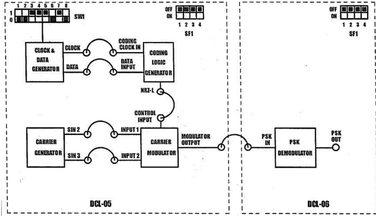
Fig 7.1 Block diagram for Binary Phase Shift Keying
