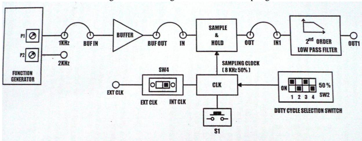
Fig. 1.2 Block Diagram for Sample and Hold
