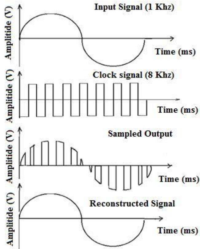
Fig 1.4 Model Graph for Signal sampling and reconstruction using sample & hold.
