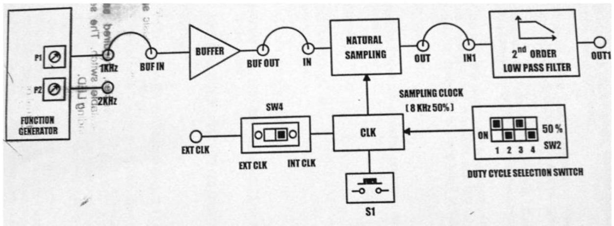
Fig. 1.1 Block Diagram for Natural Sampling
