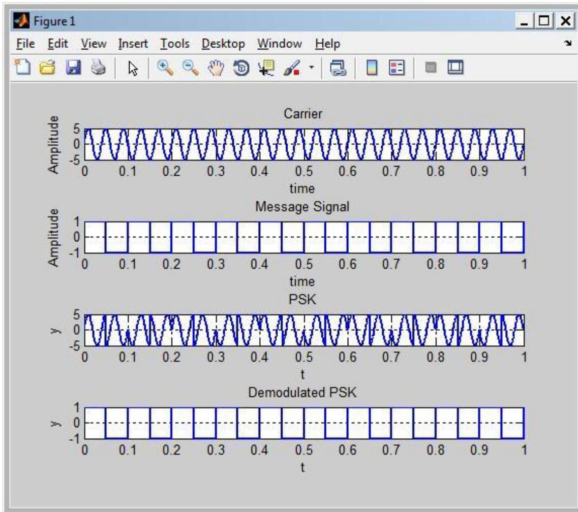
Fig 10.2 Matlab Simulation of PSK
