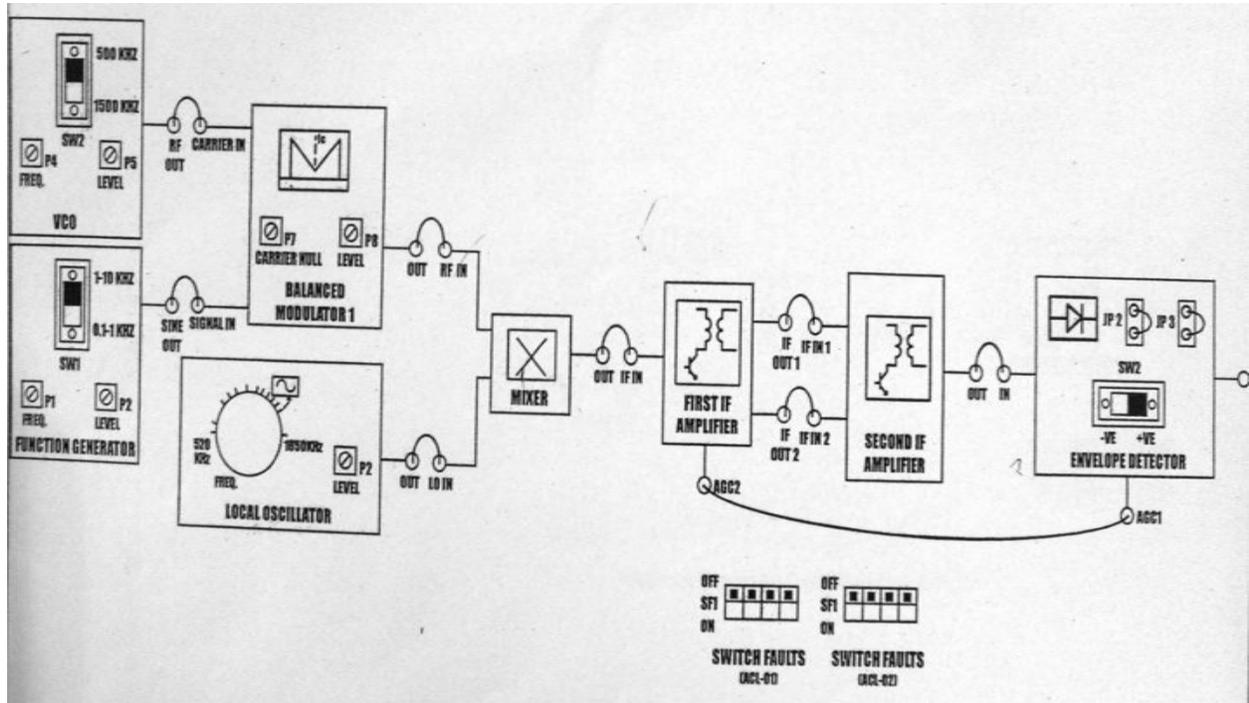
Fig. 2.1 Block Diagram for AM Modulation and Demodulation
