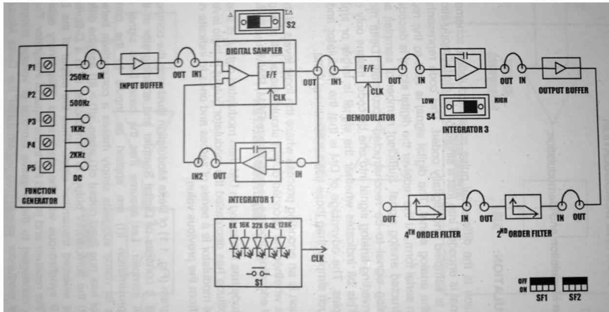
Fig 5.1a Block diagram for delta modulation and demodulation
