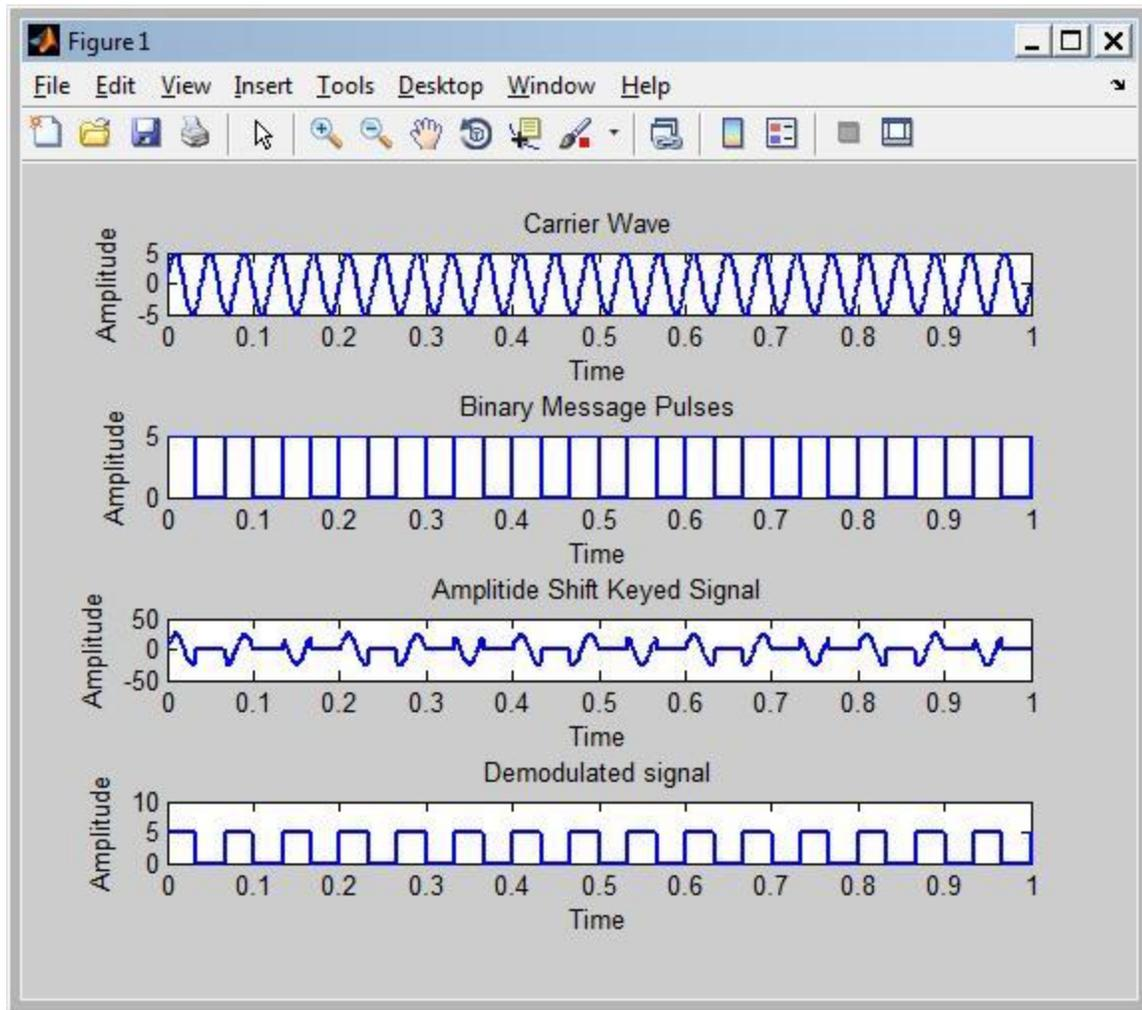
Fig 10.1 Matlab Simulation of ASK
