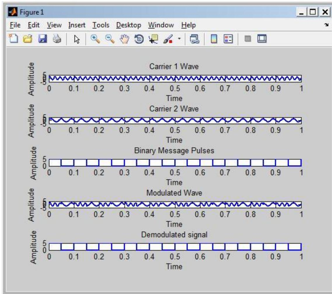
Fig 10.2 Matlab Simulation of FSK
