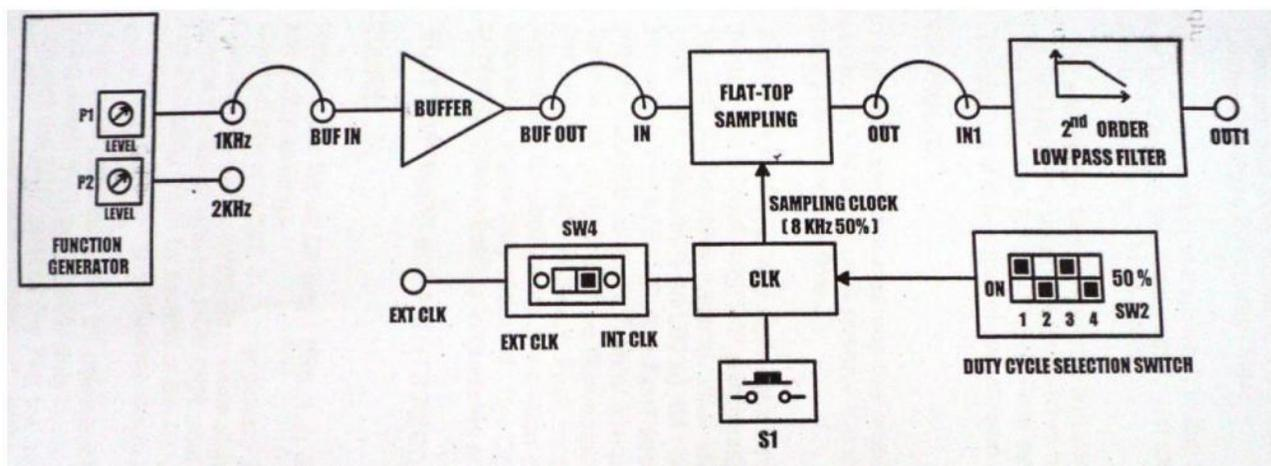
Fig. 1.3 Block Diagram for Flat Top Sampling
