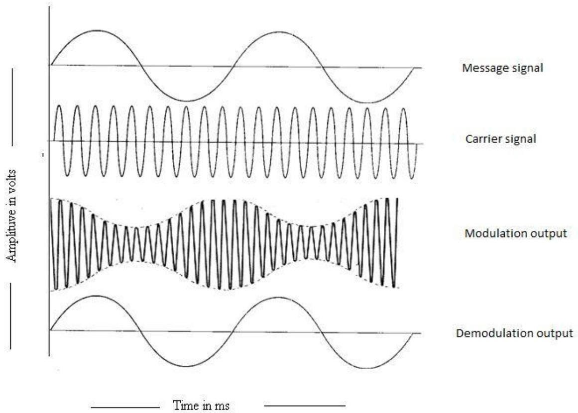
Fig. 2.1 Model Graph for AM Modulation and demodulation.
