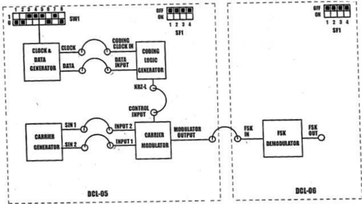
Fig 6.1 Block diagram for Frequency Shift Keying
