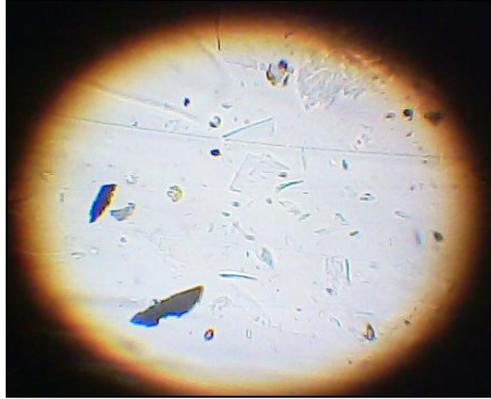
Fig.3: Several defect features occurred on my apatite samples. These defects lead to possible errors in the counting.
